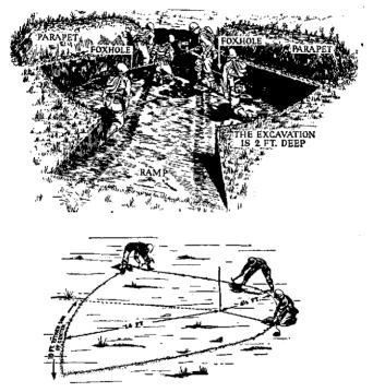
Figure 31. Fan type emplacement for 57-mm antitank gun.
