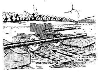
Figure 40. Method of placing gun on raft by use of sandbag ramp.
