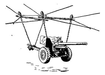
Figure 45. Aerial cableway showing movement of 57-mm antitank gun by double-cable crossing.
