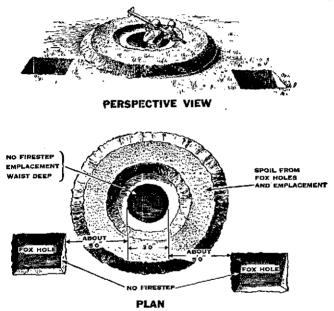
Figure 32. Pit fox-hole type emplacement for rocket launcher.
