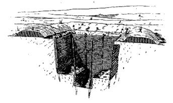
Figure 38. Revetment of two-man fox hole.
