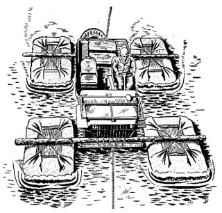
Figure 41. Flotation of 1/4-ton truck on brush raft.
