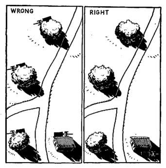
Figure 5. Vehicles concealed during a halt.
