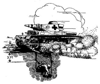
Figure 27. One-man fox hole affording protection against tanks.
