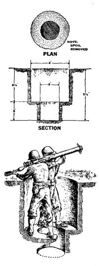
Figure 33. Pit type emplacement for rocket launcher.
